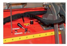
The AC 10 automatic chain tensioner maintains optimal saw chain tension at all times. The chain can be conveniently replaced after releasing chain tension with the lever pictured – no tools required!
